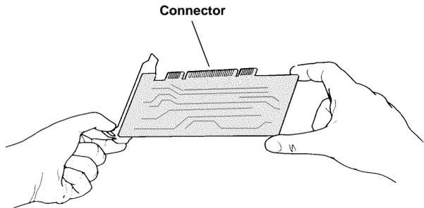
*Do not force the card. The card should fit snugly into the expansion slot.*
