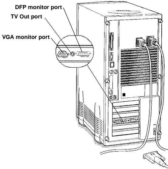
*If you have a VGA monitor, connect it to the VGA monitor port. If you have a TV monitor, connect it to the TV Out port. If you have a digital flat panel, connect it to the DFP port.*
