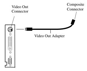
5 If you are using S-Video attach one end of an S-Video cable to the S-Video Out connector of the RADEON 7000 MAC EDITION and the other to the S-Video In connector of your VCR. If you are using Composite connect the supplied Video Out Adapter to the S-Video connector of the RADEON 7000 MAC EDITION. Then attach one end of your Composite cable to the Composite connector and the other end to the Composite In of your VCR (See diagram above).
