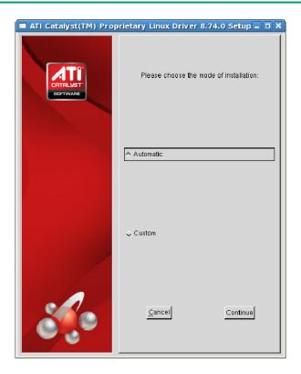
5 Select *Automatic* and click **Continue**. The ATI Catalyst<sup>TM</sup> Proprietary Linux Driver is now installed, and the Installation Complete Dialog box will be displayed.
