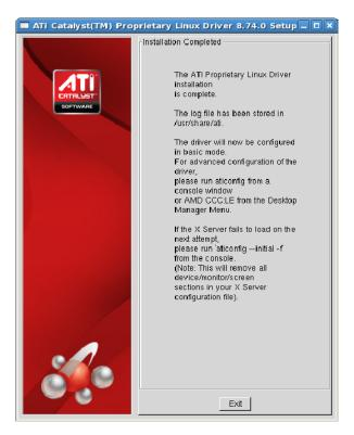
6 Click **Exit** to close the ATI Catalyst<sup>TM</sup> Proprietary Linux Driver Installer.
