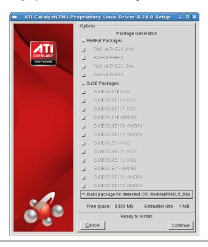
5 Select the distribution package to be generated and click Continue. The package generation will start and the Package Generation Completed dialog box will be displayed.
