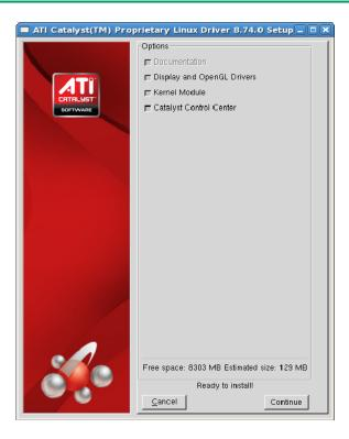
6 Select the driver components to be installed and click **Continue**. The ATI Catalyst™ Proprietary Linux Driver is installed, and the Installation Complete Dialog box will be displayed.
