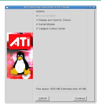
6 Select the driver components to be installed and click **Continue**. The ATI Proprietary Linux Driver is installed, and the Installation Complete Dialog box will be displayed.
